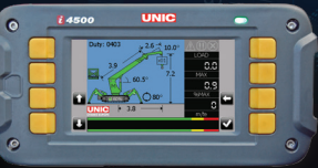
Full safe load indicator
