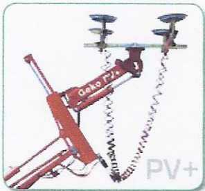
The Geko PV+ arm allows panels weighing up to 175kg to be picked up and tilted 180° for overhead and ceiling installation up to 3m high.
